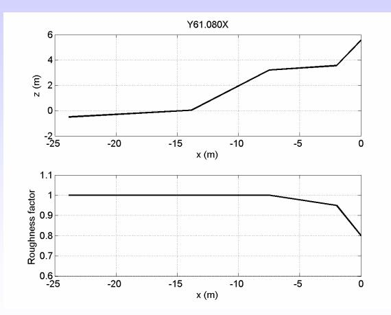
Schematized dike profile and roughness factor
