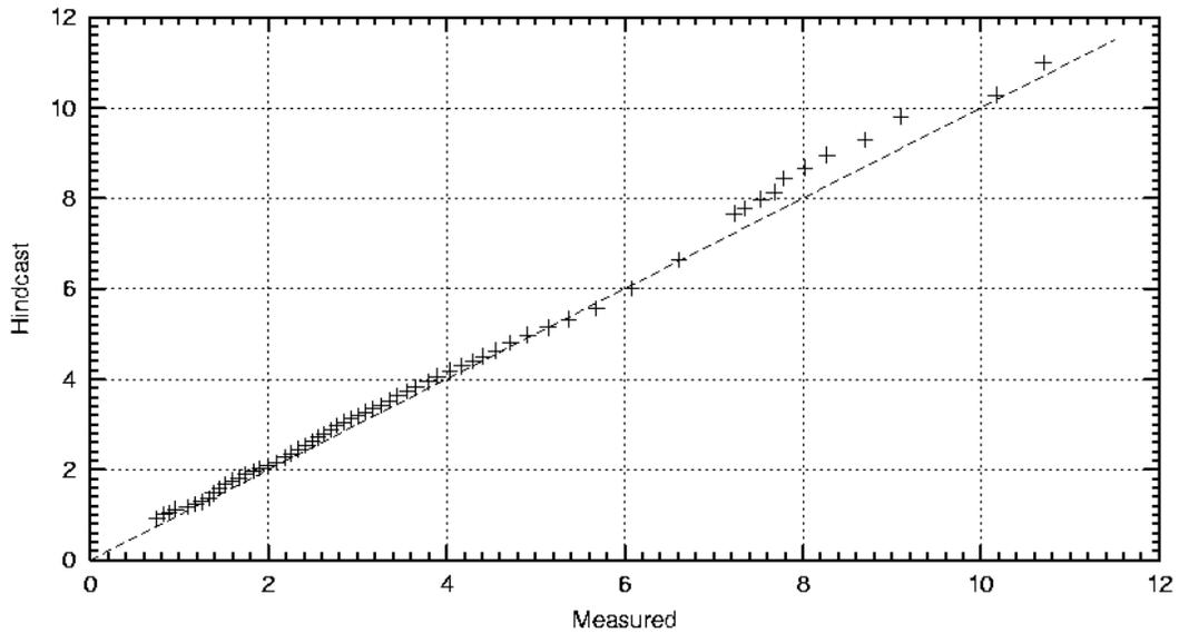
Figure 8. Quantile-Quantile Plot for Hm0 (m) at NDBC Buoy 46006 (40.84° N 137.49° W)
