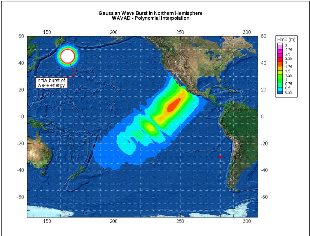
Figure 3. Wave Height Contours for Wavewatch III Results for QUICKEST Propagation Scheme
