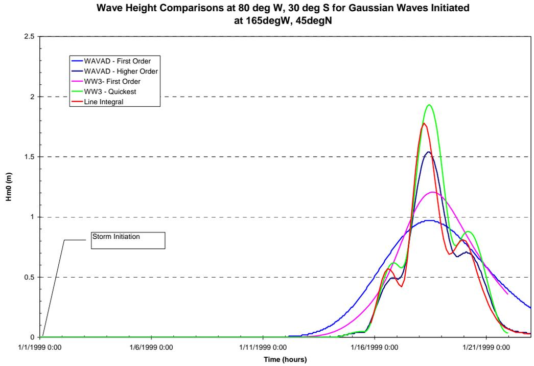
Figure 4. Inter-comparisons of Significant Wave Height at 30°S, 80°W
