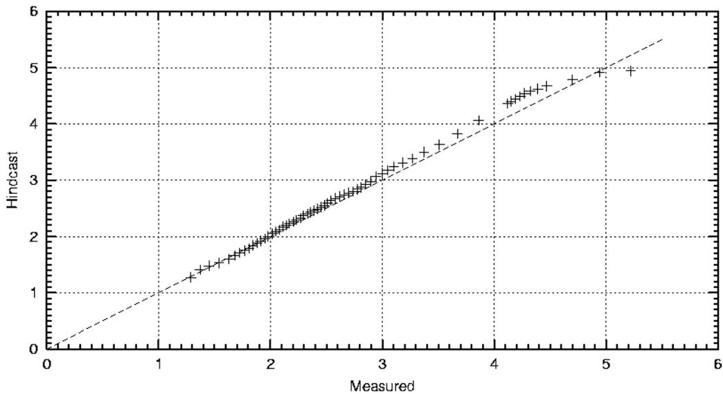
Figure 9. Quantile-Quantile Plot for Hm0 (m) at NDBC Buoy 51002 (17.14° N 157.79° W)
