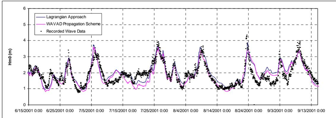
Figure 10. Sample Time Series Comparison [Buoy 45059 37.98°N 130.00°W]
