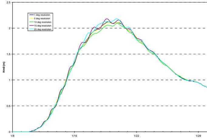
Figure 9. Hindcast Significant Wave Height at 80°W,30°S for Varying Numbers of Wave Rays
