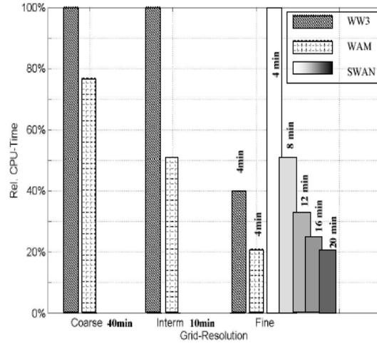
Figure 3: Relative CPU times for the models for January 2002 Bomb, with time steps indicated.
