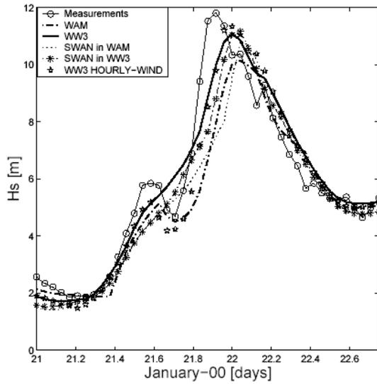
Figure 6: Hindcast and measured  $H_s$  at PANUKE location for Superbomb.
