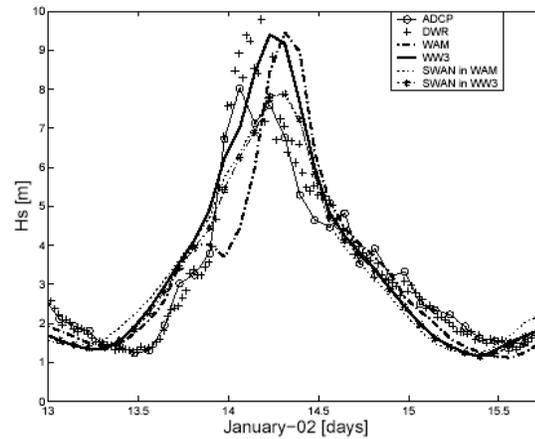
Figure 4: Hindcast and measured Hs at the ADCP – DWR location for January 2002 Bomb.
