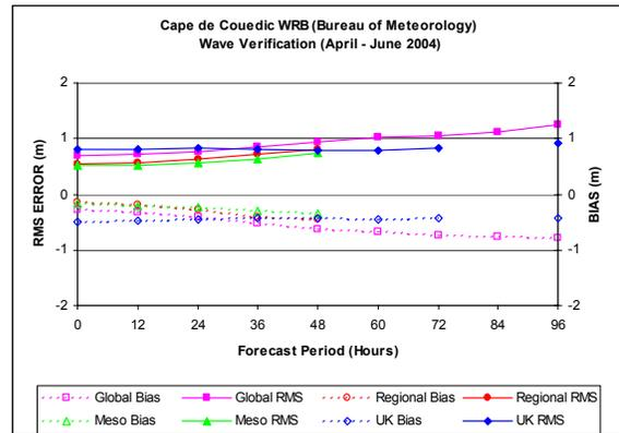
Fig. 5 Verification statistics for global, Australian Region, Australian meso-scale and UK global wave models against observations at Cape du Couedic for the period April – June 2004.
