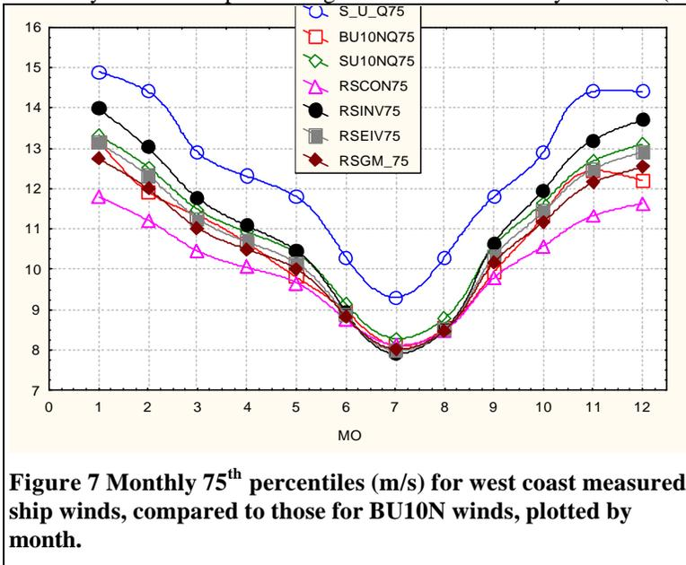
**Figure 7 Monthly 75<sup>th</sup> percentiles (m/s) for west coast measured ship winds, compared to those for BU10N winds, plotted by month.**
