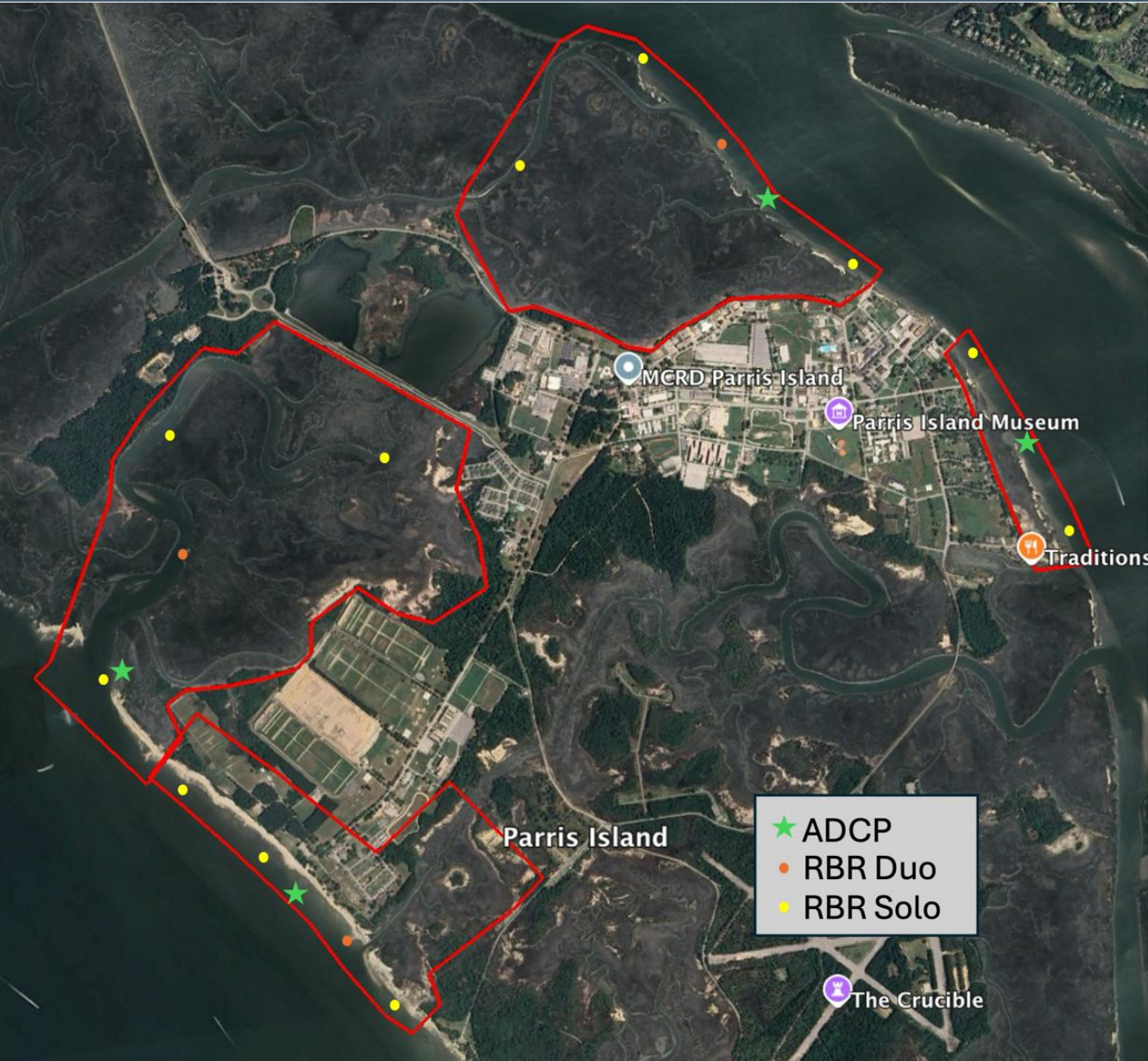
Pressure (RBR) and velocity profilers (ADCP)
