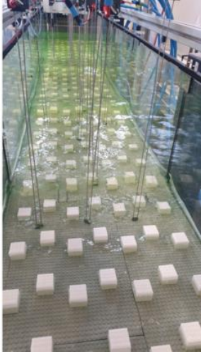
Rough seabed surfzone experiments in the CASH flume (SEATECH/MIO, Toulon) : LEGOLAS & COCODYROCK experiments
