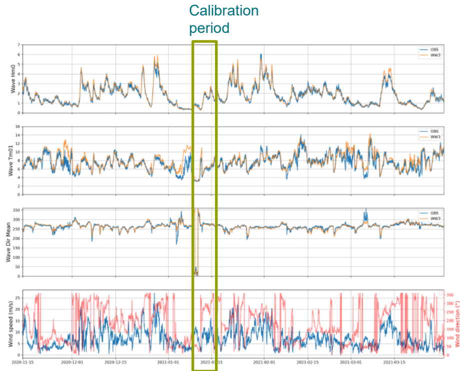
Significant wave height ( Hm0 ) (top) and mean period ( Tm01 ) (middle) at T2-6 measured (in blue) and simulated by NORGASUG( WW3 in orange), Wind speed (blue) and direction (red) measured at Saint-Clement-des-Baleines (bottom) during LEG1 and LEG2
