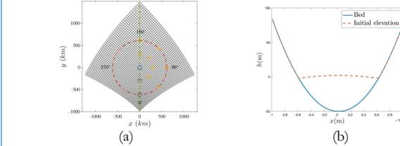
(a) Bathymetry of bowl case in OCCS with three stationary locations (b) Initial condition at x=0m
