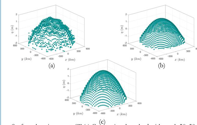
Surface elevation at t = 6T (a) Conventional method with mesh 50x50 (b) subgrid method with mesh 50x50 (c) Analytical solution
