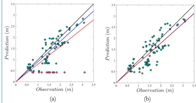
Peak water level comparison between observations and coarse grid simulations: (a) Conventional and (b) Subgrid method
