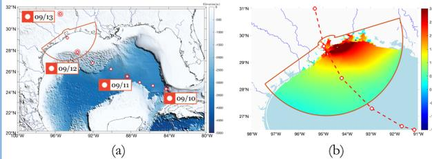
Example case for Ike (a) Hurricane setup (b) Simulation result for maximum surface elevation
