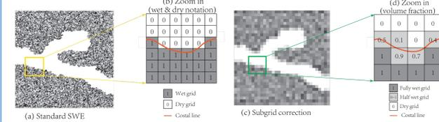
Wetting and drying methods (a) Standard method (c) Subgrid method
