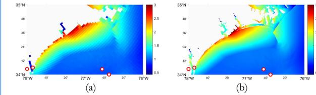
Maximum Surface Elevation for Hurricane Florence 2018 at Onslow Bay, NC (a) Coarse grid (~4.3 km) (b) Fine grid simulation (~0.5 km)
