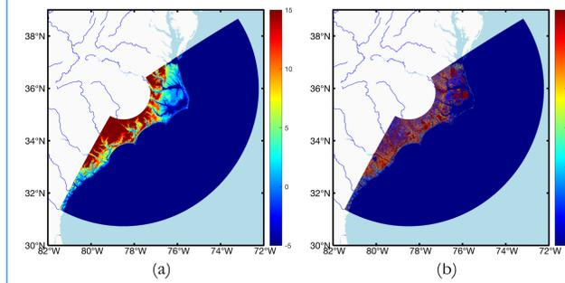
Input data represented by high-resolution subgrid resolution (mesh size 13567 × 22784) (a) Ground surface elevations (m relative to NAVD88) generated from NOAA Digital Coast with finest ~5m (b) Manning coefficients corresponding to different land cover based on National Land Cover Database 2019 with 30 m resolution
