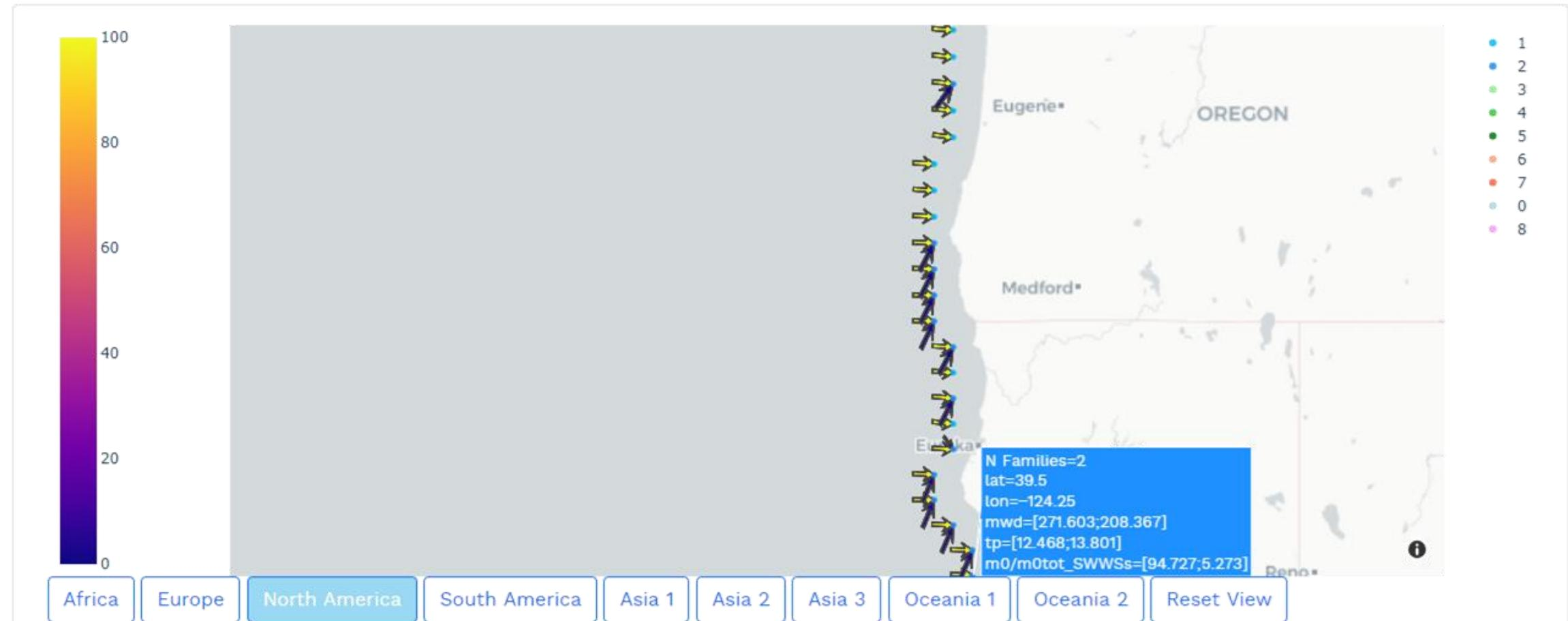
The color identifies the relative energy of each family, it is expressed in percentage,  $\frac{m_{0Wsys_i}}{m_{0Wsys_{tot}}}$ . The size of the arrow represents the time averaged  $T_p$ , whereas the number of the arrow are the number of wave systems that exist in that location, the direction of the arrow represent the time averaged  $MWD$  where the wave systems come from.
