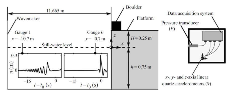
Experimental setup showing the wave flume on the left and the "smart" boulder internal instrumentation on the right (Ecole Centrale de Marseille)
