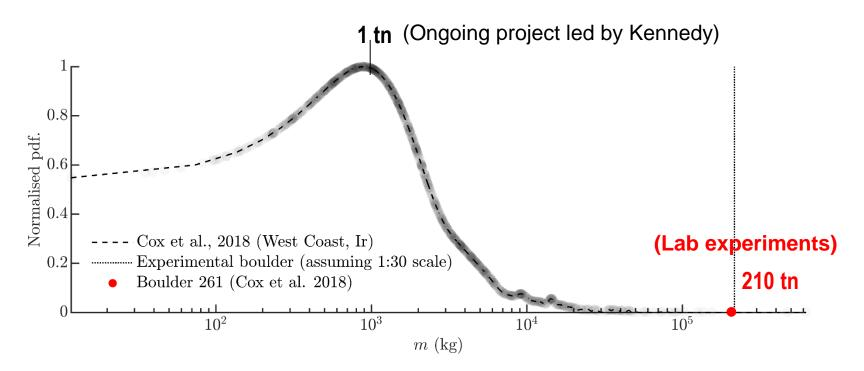
Boulder mass probability distribution (normalised) on the Irish west coast as measured by Cox et al. (2018). The mass of the model boulder, at prototype scale (1:30), is given by the dotted line and boulder 261 is denoted by the red dot.
