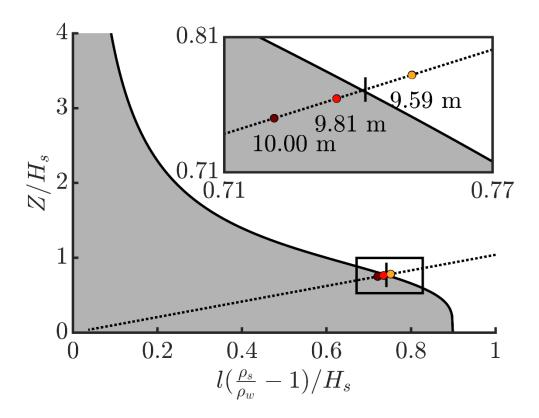
Position of the experimental waves in the initiation of motion space derived by Kennedy, Cox & Dias (2021)
