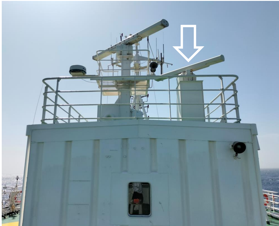
Photo of the radar antenna JRC JMA-9122-6XA of the R/V Academic Ioffe
