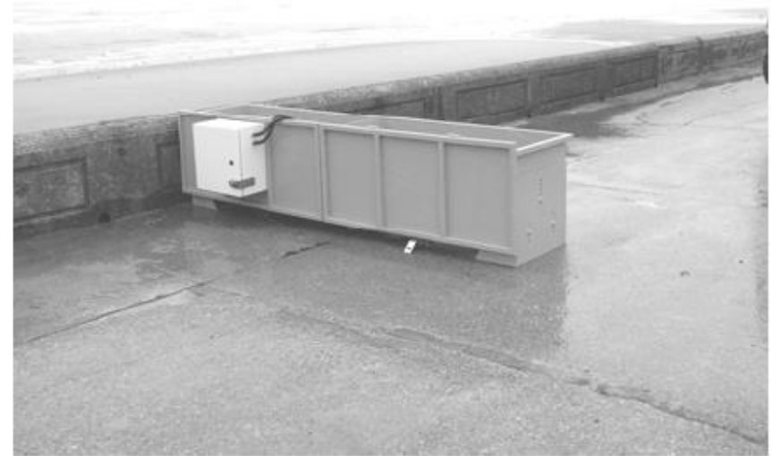
The seawall at Anchorsholme, and the overtopping tank in position
