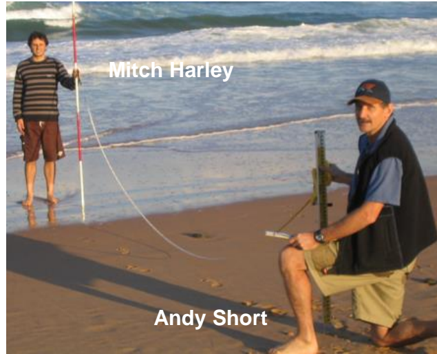
Historical surveying using Emery method
