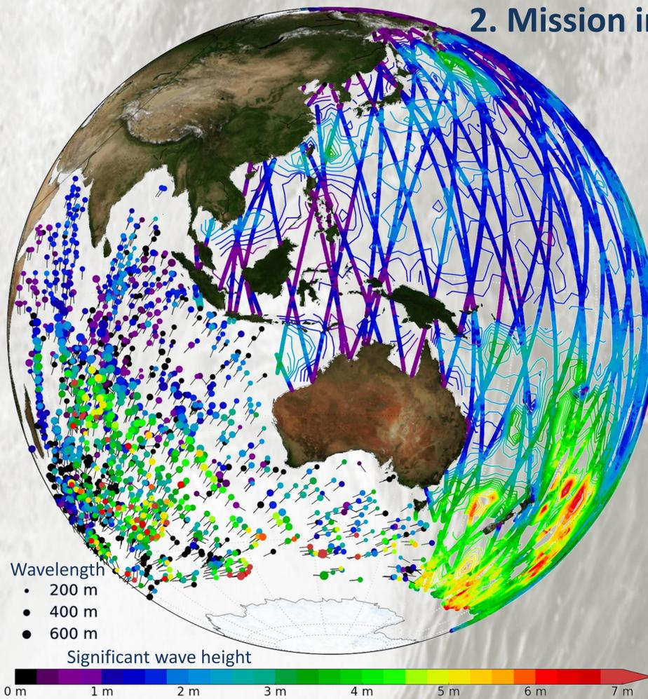
Left: SAR-derived swell conditions ; Right: Altimetry-derived along-track and gridded (contours) significant wave height
