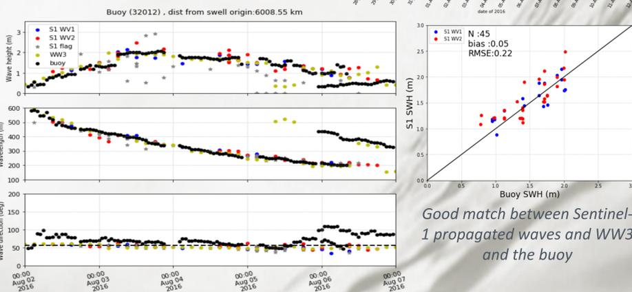
Significant wave height, peak wavelength and peak direction given by the L3 CMEMS SAR products at the buoy location compared to the WW3 model and in situ measurements
