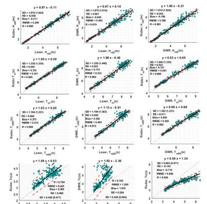
Figure 6: Passing Bablok non-parametric regression between the significant wave heights ( $H_{m0}$ ), mean wave periods ( $T_{m01}$ ), zero-crossing wave periods ( $T_{m02}$ ), and crest wave periods ( $T_c$ ) of the Laser, the Radar and the DWR.
