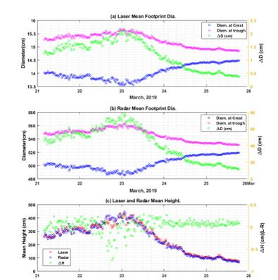
Figure 5: (a) Laser mean footprint diameter at wave crests and wave trough; (b) Radar mean footprint diameter at wave crests and wave trough; (c) Laser and DWR mean wave height.
