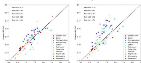
Figure 6. Comparison of observed breaking wave height ( $H_s$ , x-axis) versus: (left) predicted wave height based on downscaling and surf height prediction; (right) a naive prediction using modelled wave height at closest grid cell ( $H_0$ ). Surf prediction outliers occur at Looe (LST), where strong tidal variations affect incident energy and are not represented in the driving model, and Doolin, where beach profile is relatively steep and has a stepped morphology (Poate et al. 2017)
