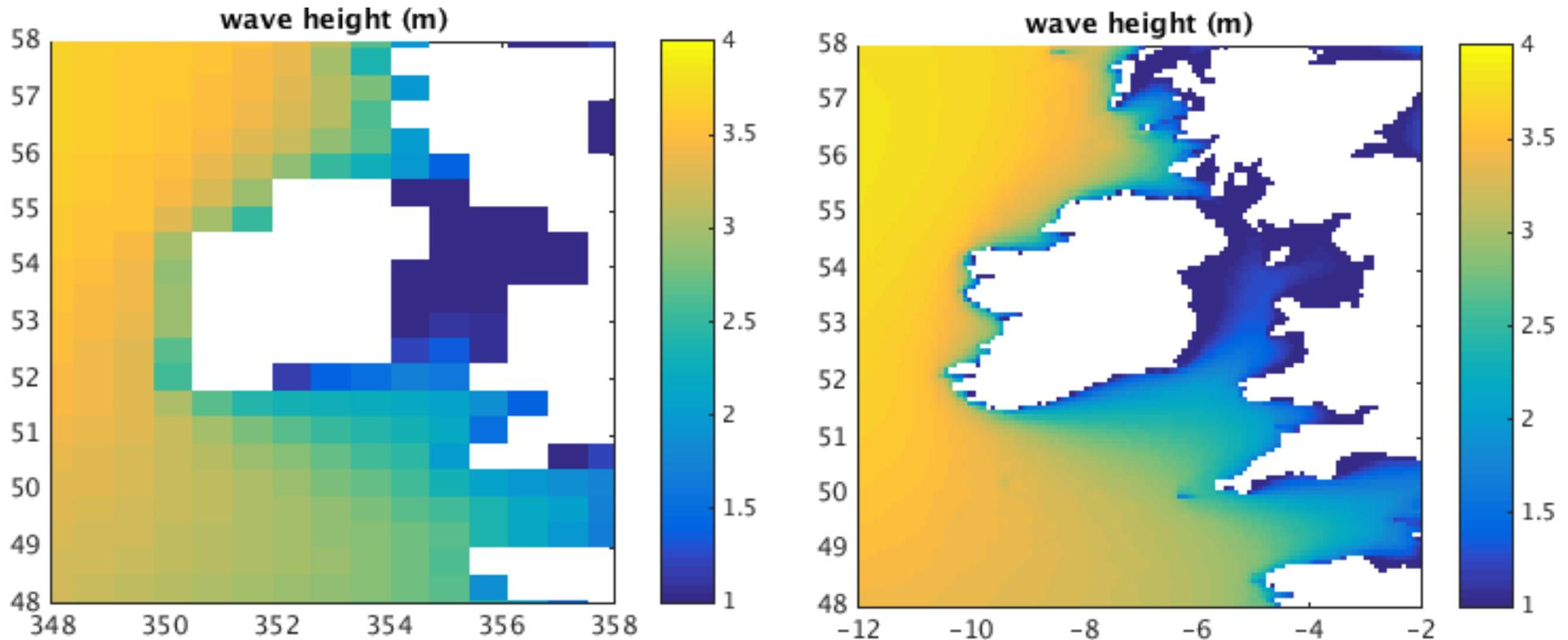
Global model (left) resolution  $\sim 0.83^\circ$  High resolution (right) resolution  $\sim 12\text{km}$ . 30 year means for historic run 1970 – 1999
