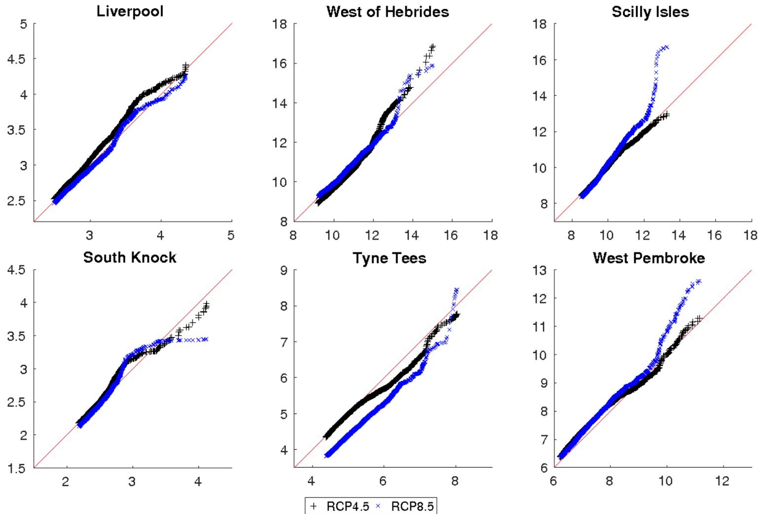
Quantile-Quantile plots of the top 1% of significant wave height for six sites. By plotting the historic (x-axis) against 2 futures (y-axis) we can see divergence where the extreme wave climate changes in future.
