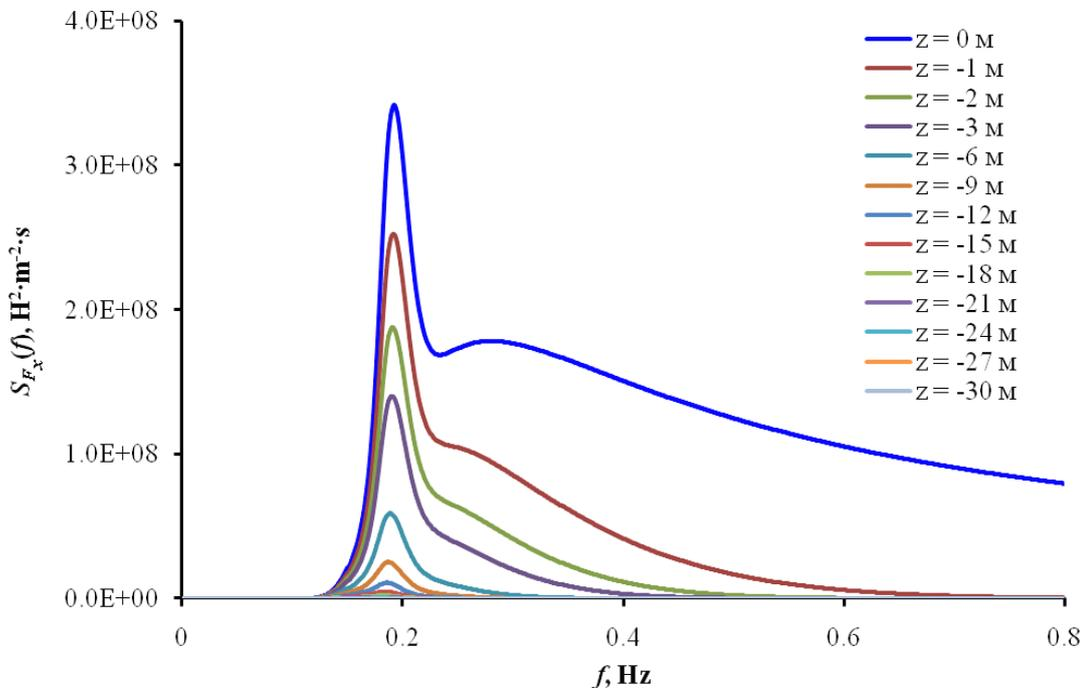
**Fig. 6.** Spectral density of horizontal component of wave induced force for monthly loading case
