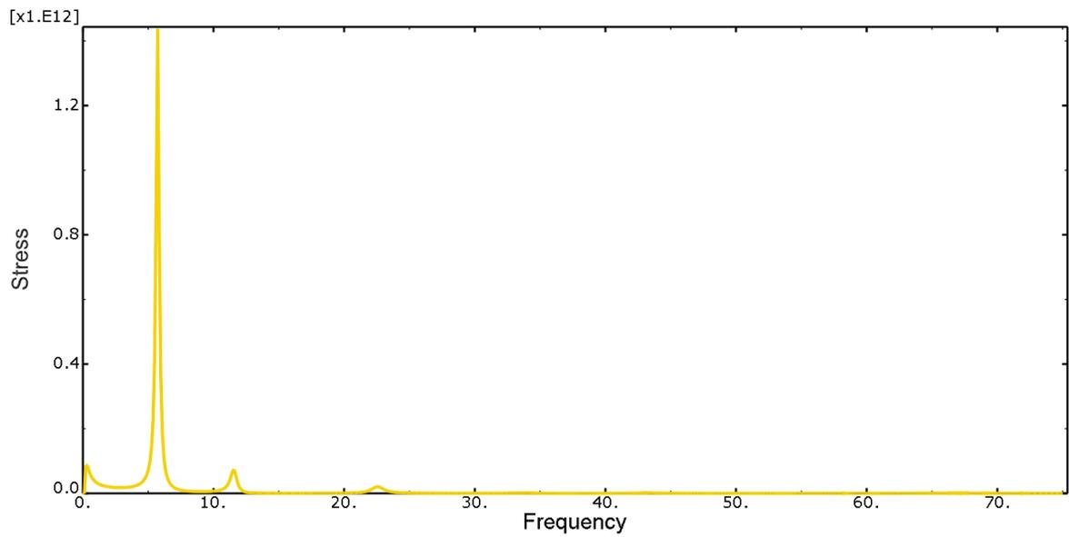
**Fig. 8.** Envelope of spectral densities  $S_{\sigma_{waves}}(f)$  of stresses in buoy's concrete body for monthly loading case
