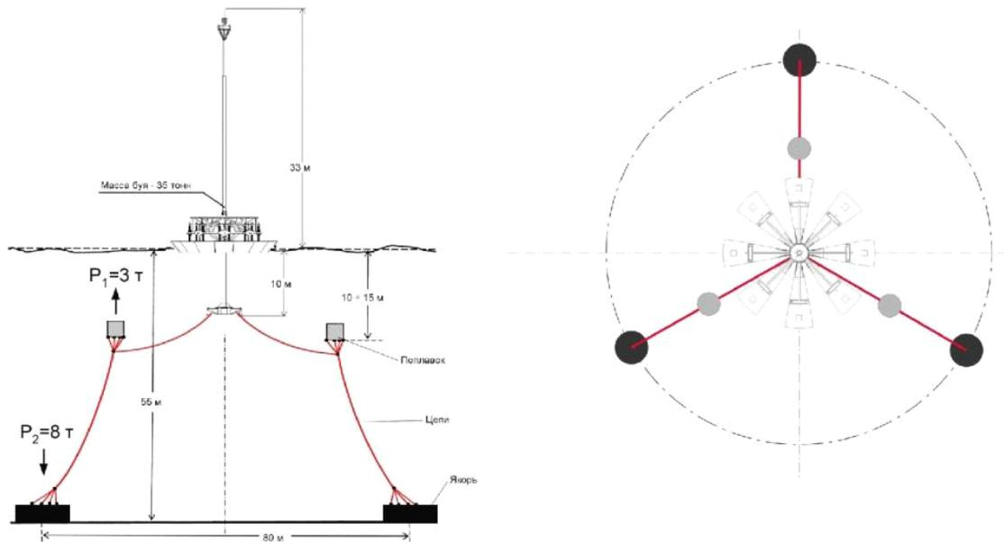
**Fig.10.** The anchor system of the concrete spar buoy
