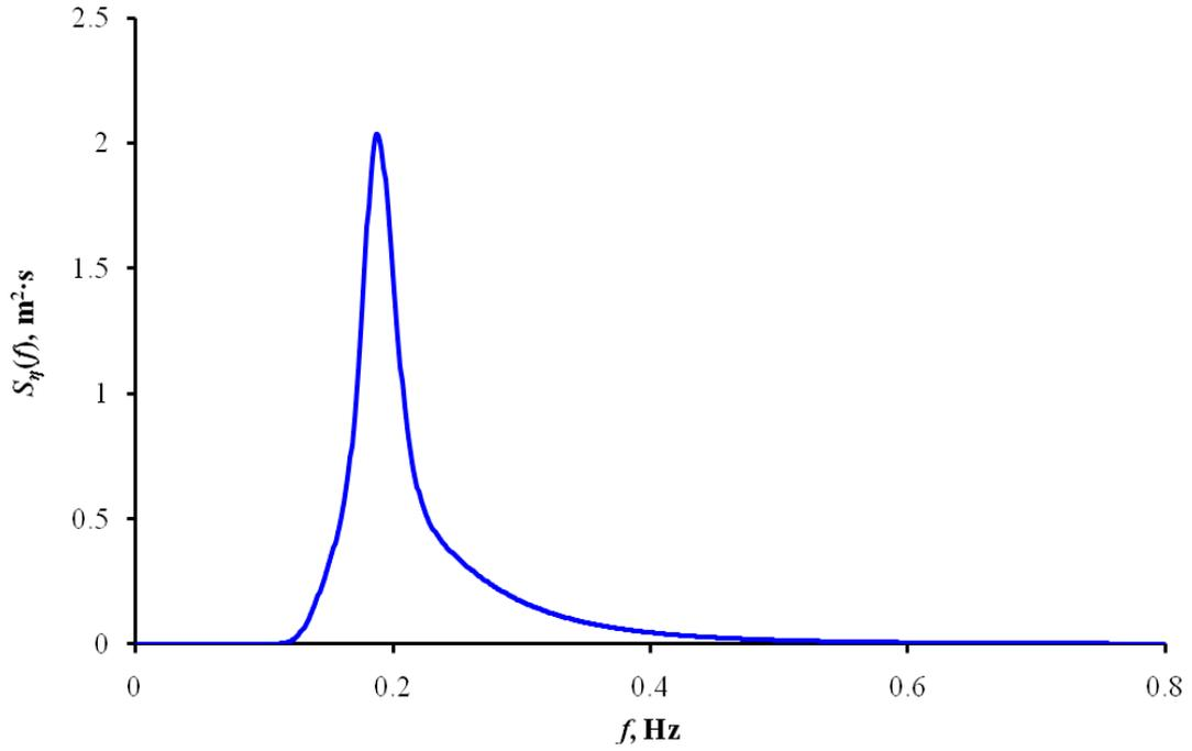
**Fig. 5.** Spectral density of sea surface elevation for monthly loading case
