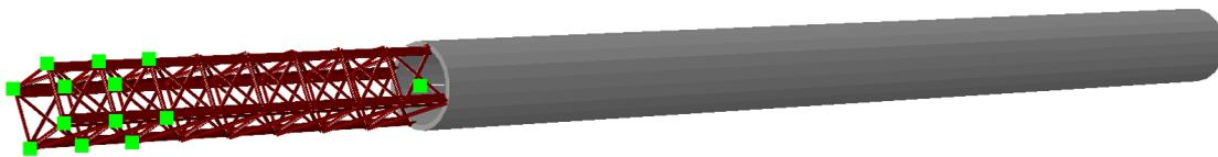
**Fig. 7.** Buoy's numerical model (point masses are shown with green squares)
