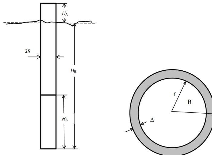
**Fig. 4.** The project of the concrete stabilized spar buoy.
