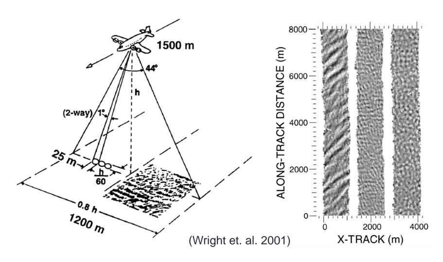
SRA resolve waves equal or longer than 50m (~ 0.17 Hz)
