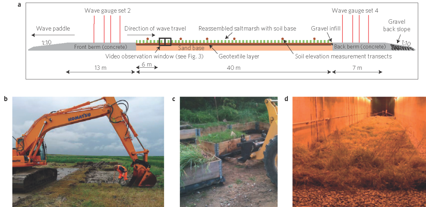
Figure 1 | Experimental set-up and photographs of excavation. a , General experimental set-up in the wave flume, with position of recording equipment relevant to reported results. b , Excavation of marsh blocks, northern German Wadden Sea ( 53^{\circ} 42.754' \text{ N} , 7^{\circ} 52.963' \text{ E} ). c , Marsh blocks with Elymus vegetation cover before positioning in the flume test section. d , Reassembled salt marsh inside the 5-m-wide flume, looking towards the wave generator; lamps are mounted at about 3 m above the soil surface.
