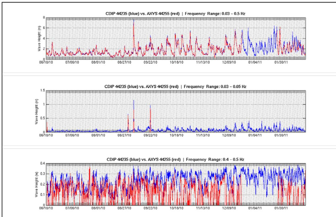
Figure 4. Evaluation of two co-located wave measurements over time, for total (top panel), low frequency (middle panel), and high frequency (lower panel) ranges. The CDIP 44235 is the Environment Canada Datawell Directional Waverider, AXYS 44255 is the 6-m MONAD hull and the TriAxys sensor. Note results were also compared to the 6-m NOMAD hull using the Environment Canada operational strapdown accelerometer payload. All figures refer to the two buoys indicated here.
