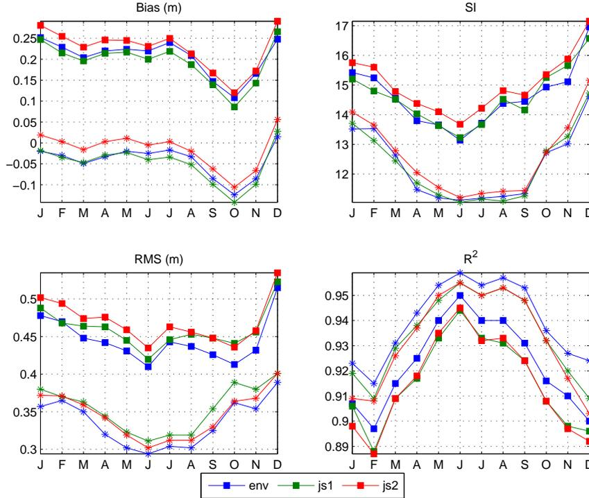
Fig. 3: Global monthly model error statistics against the ENVISAT (env), Jason-1 (js1) and Jason-2 (js2) altimeter for 2009. Bias (m), Scatter Index (%), rms error (m) and  $R^2$  (-). Solid squares for old model (as in Fig. 2a), asterisk for new model (as in Fig. 2b).
