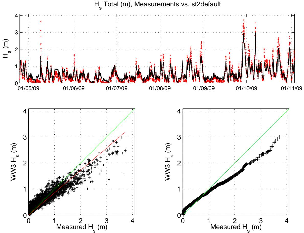
Fig. 4: Wave height validation for Great Lakes buoy 45007 for 2009. Upper panel is time series, with mode as black line and observations as red symbols. Lower left panel is scatter plot, with linear regression line in green. Lower right plot is quantile-quantile (qq) plot comparing pdfs of model and observations. Present operational model based on Tolman and Chalikov (1996) physics.
