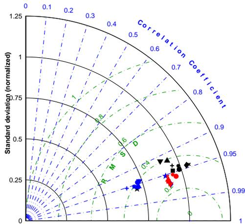
Fig. 6: Taylor diagram for wave heights for deep water buoys in the Great Lakes for 2009 using analysis wind fields of Schwab and Morton (1984). Symbols identify individual buoys. Colors identify model. Blue: Tolman and Chalikov (1996) physics. Red: Ardhuin et al. (2010) physics. Black: second generation GLERL-Donelan model (Schwab et al., 1984).
