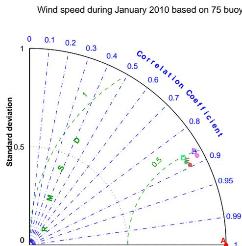
Fig. 1: Taylor diagram for various global wind field errors for January 2010 based on wind speed observations at 75 buoys. A represents the observations, B-E represent various wind field sources.
