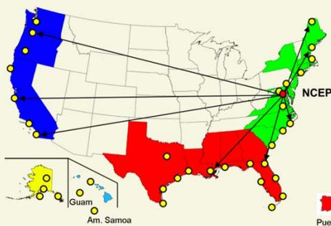
Figure 3: Concept of decentralized computing of nearshore wave and circulation model guidance. NCEP provides central support and forcing data, but each coastal WFO (yellow dots) in each of the NWS regions (colors) runs its own local model.
