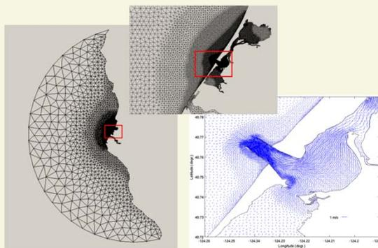
Figure 6: Unstructured grid for the coupled computation of waves and current at WFO Eureka (Northern California). Bottom right-hand panel shows vector plot of tidal currents through the Humboldt Bay harbor entrance.
