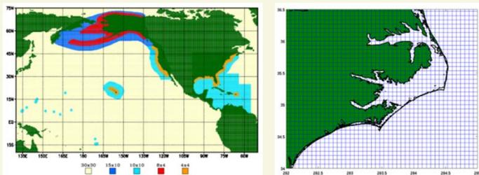
Figure 2: Left: Present Multigrad WWIII two-way nested mosaic computational grid, showing a global grid resolution of 30x30 arc min, and detailed regions with resolutions of down to 4x4 arc min. Right: Shelf-scale 4x4 arc min grid over the domain of responsibility of WFO Morehead City, showing the relative coarseness of the grid compared to coastal features.
