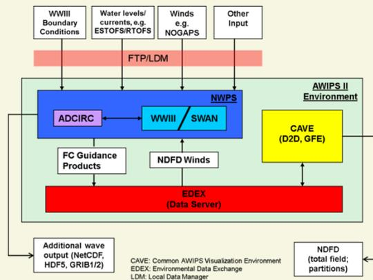
Figure 4: Schematic architecture of the NWPS system within the AWIPS II structure. Significant components are the EDEX data server for main data storage, the CAVE visualization environment and the NWPS wave and circulation modeling module.
