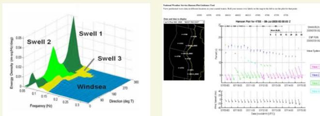
Figure 5: Left: Example of a directional wave spectrum decomposed into a number of partitions (Tracy et al. 2007). Right: Gerling-Hanson plot showing the time evolution of various wave systems in the domain of responsibility (insert).
