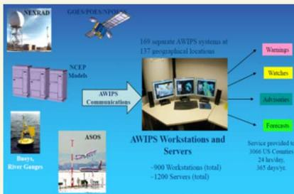
Figure 1: The Advanced Weather Interactive Processing System (AWIPS) combines various data sources including satellite, radar, weather buoy and aviation-related observations, as well as numerical model results (model guidance) from NCEP, in a single display environment for forecasters at WFOs and national centers to interpret. Based on these data, a number of products are prepared, including warnings, watches, advisories and forecasts.
