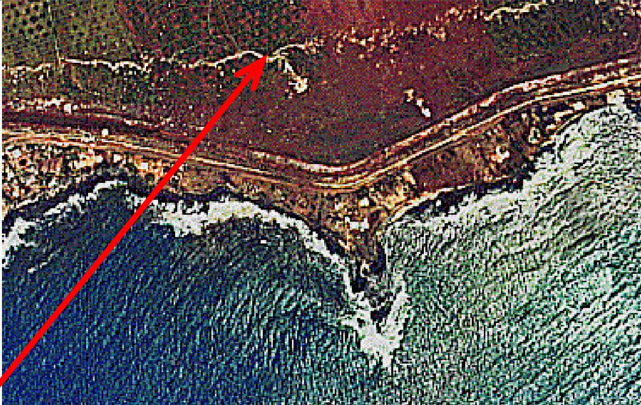
**Hurricane Iniki (1992) debris line is much further inland and higher elevation (~7m) than the 2-3 m surge.**
