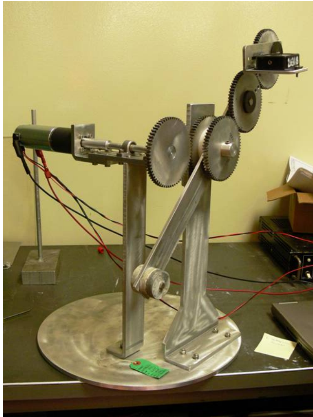
Figure 5: Desk-Top Wave Simulator (DTWS). The radius of the arm is 24 cm.
