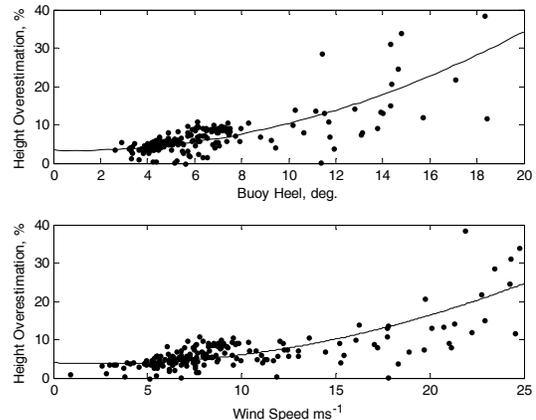
Figure 8. Same as Fig. 7, except for the 2.25-m discus buoy during the passage of Ike.
