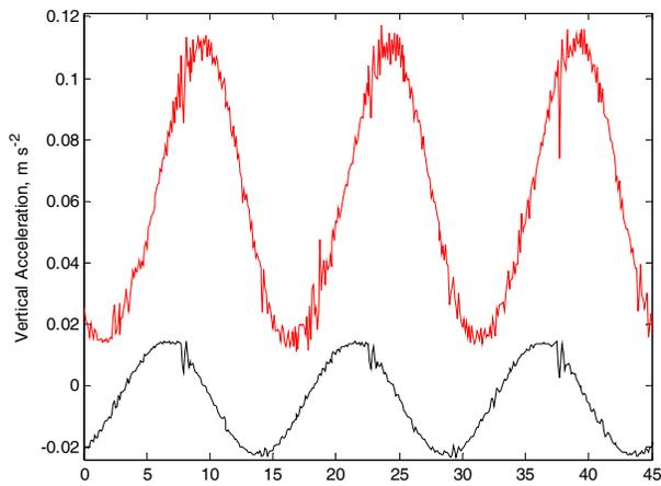
Figure 9. The measured vertical acceleration for the OWIF simulation run of a one-m amplitude wave with a period of 15 s, a maximum wave slope angle of  $8^\circ$ , and a buoy heel of  $20^\circ$ . The Crossbow 1D accelerometer is shown in red and the Hippy 40 is in black.
