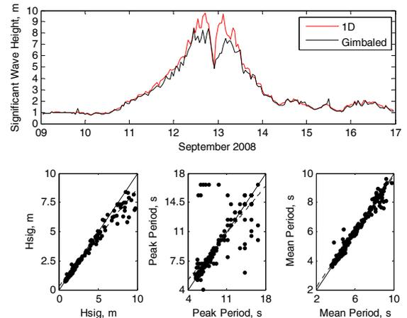
Figure 4. The same as Fig. 2, except for the 2.25 m buoy for the period from September 9<sup>th</sup> through September 17<sup>th</sup> 2008 during the passage of Ike.
