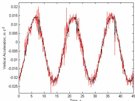
Figure 10. The measured vertical acceleration for the OWIF simulation run of a one-m amplitude wave with a period of 15 s, a maximum wave slope angle of  $8^\circ$ , and a buoy heel of  $20^\circ$ . The mathematically gimballed Crossbow accelerometer is shown in red and the Hippy 40 is in black.
