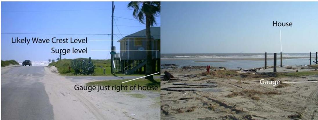
Figure 5. The same location at Crystal Beach, Texas before and after Hurricane Ike. The USGS surge gauge GAL-1 was located just to the right of this house. Note the complete removal of the protective dune fronting the island. Photos courtesy USGS.
