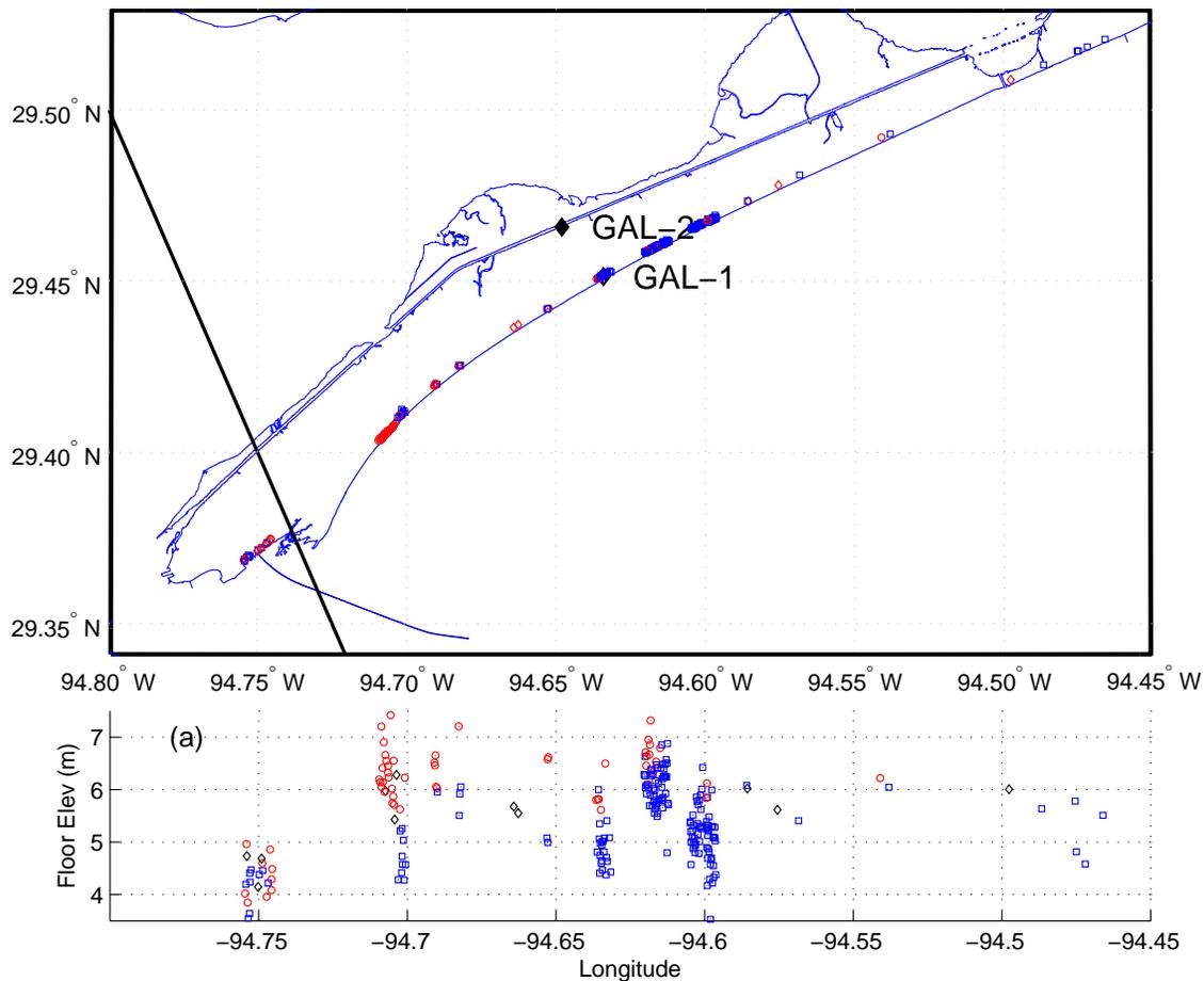
Figure 9. Survival and destruction of houses 0-150m from the Gulf of Mexico. (Top) Surveyed houses; (bottom) elevations vs destruction. (○) Surviving Houses; (□) Completely Destroyed; (◇) Surviving with wave damage.
