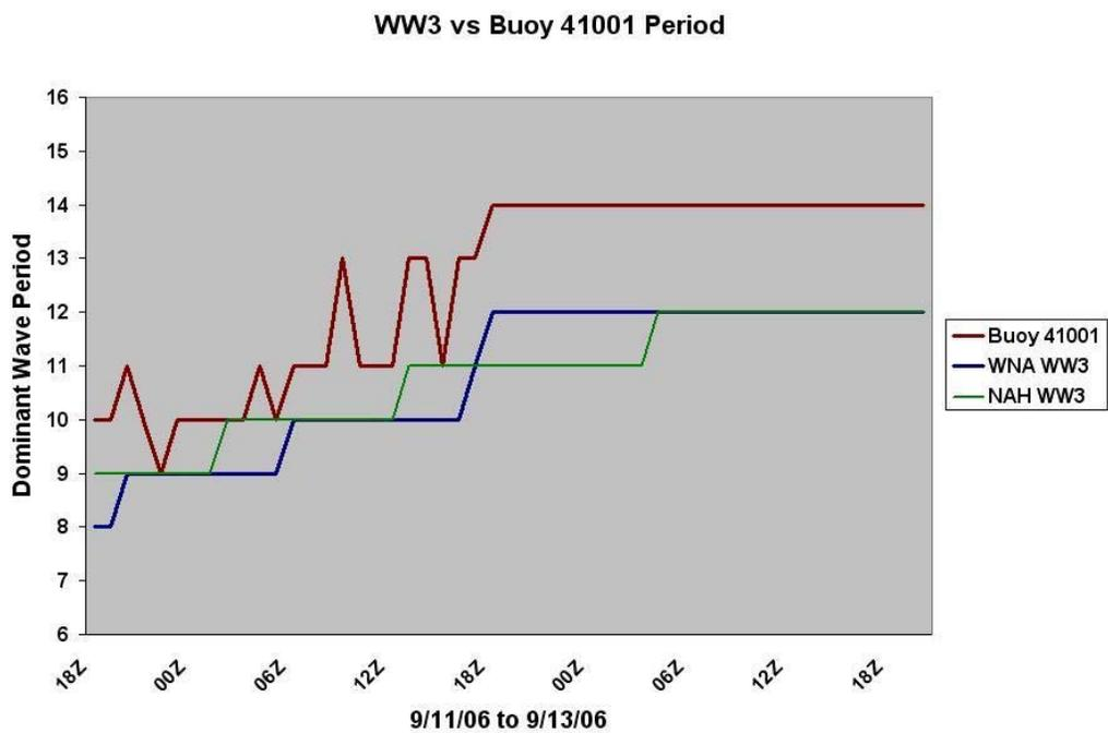
**Figure 10.** Observed and modeled dominant wave period (s) at buoy 41001 from 11-13 September 2006.
