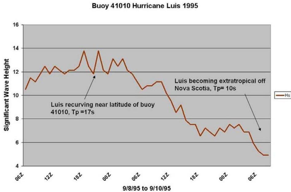
**Figure 3.** The swell event associated with Category 4 Hurricane Luis at Outer Canaveral buoy 41010, showing a peak in long period energy when the storm was near the latitude of the buoy, and then a steady drop as the storm recurved towards the Canadian Maritimes. This demonstrates a typical long period swell event for Florida associated with a tropical cyclone. Significant wave height (ft) plotted from 8-10 September 1995.
