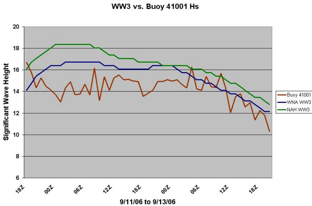
**Figure 9.** Observed and modeled significant wave heights (ft) at buoy 41001 offshore Cape Hatteras, North Carolina from 11-13 September 2006.
