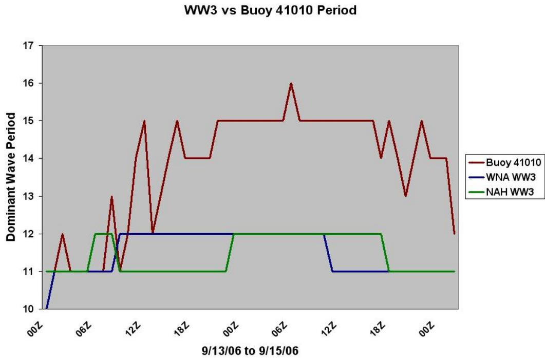
**Figure 8.** Observed and modeled dominant wave period (s) at buoy 41010 from 13-15 September 2006.
