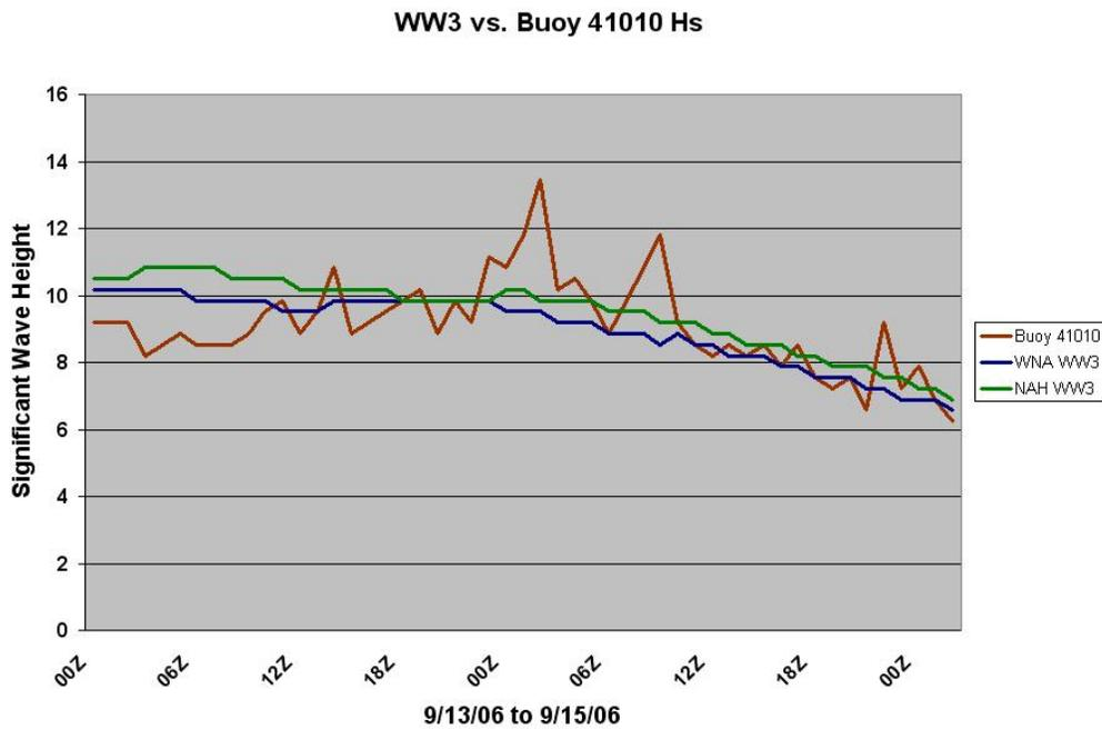
**Figure 2.** Observed and modeled significant wave heights (ft) at buoy 41010 offshore Cape Canaveral, Florida from 13-15 September 2006.
