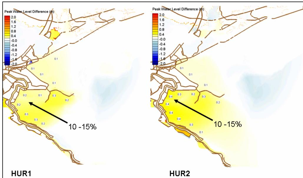
**FIGURE 4 – DIFFERENCE IN PEAK SURGE LEVEL BETWEEN FUTURE AND BASE CONDITIONS**
