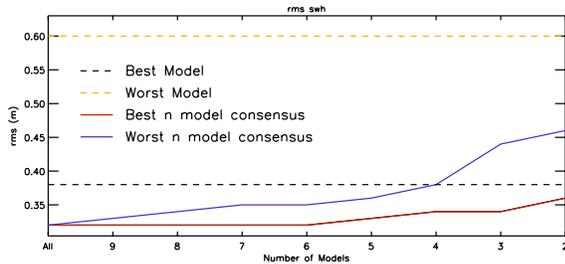
FIG. 4. 24 hour forecast  $H_s$  RMSE for PWBC as a function of the number of component models in the consensus. The best and worst n models are defined according to their RMSE. The RMSE of the best and worst individual models are included for reference.
