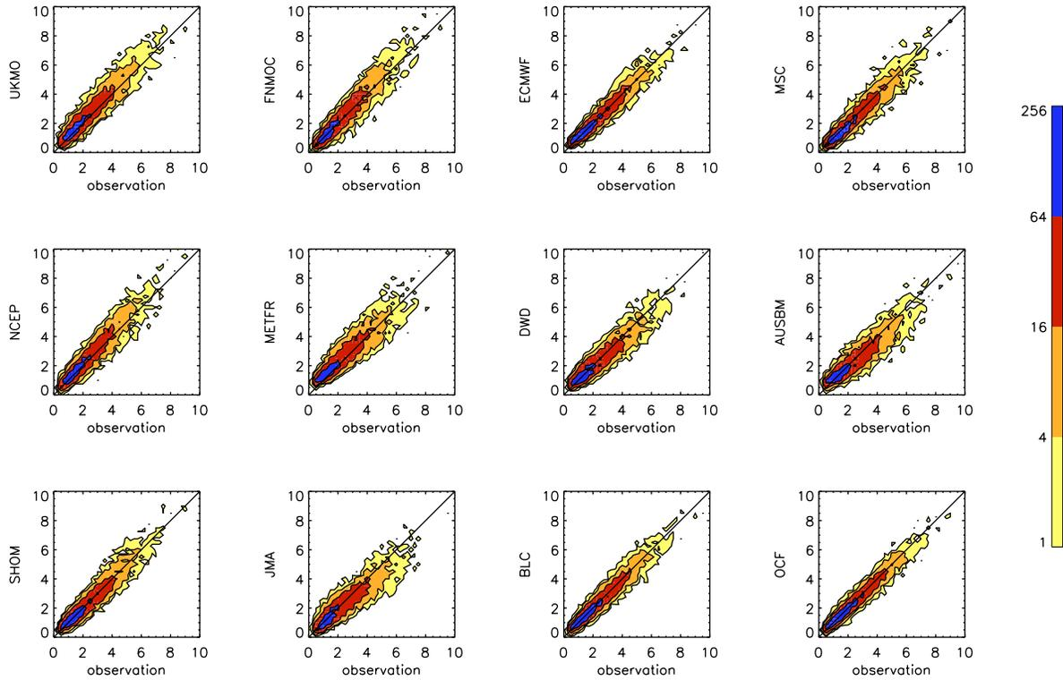
FIG. 2. Scatter plots of 24 hour forecast  $H_s$  for all raw models and BLC and PWBC (OCF) correction schemes
