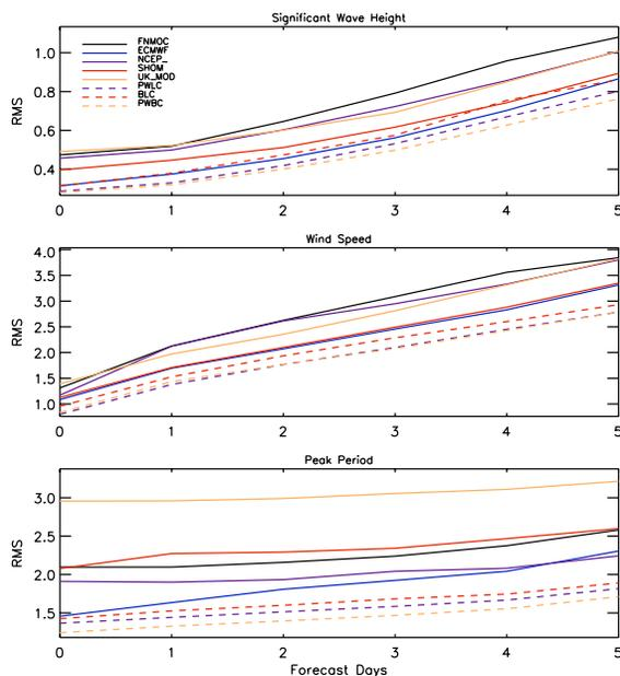
FIG. 6. RMSE growth with forecast period for model for which five day forecasts are available (FNMOC, ECMWF, NCEP, SHOM and UKMO) as well as PWBC, PWLC and BLC forecasts produced using these models.
