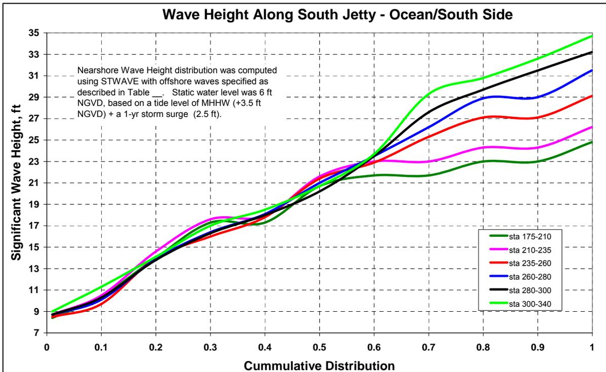
Figure 4. TOP. Cumulative distribution for wave height ( $H_{sig}$ ) at MCR. BOTTOM panel. Computed wave height along an offshore transect, (just north of white box in figure) based on variation in morphology and depth (from 25 ft – 70 ft depth). For CDF values > 0.6, much of the wave action become depth limited for inshore areas. A transient change in water level of 2 meters would have considerable effect on the above the nearshore wave environment.
