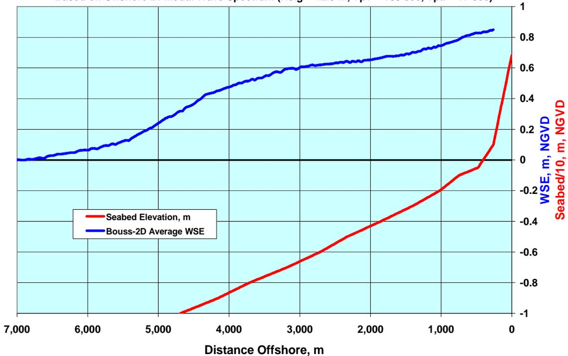
Figure 12. (TOP) Profile of seabed elevation and time-averaged WSE along “black-dashed line” (figure 10) for the entire model domain. The WSE was time-averaged during the  $t=2,000-3,000$  sec. The average WSE becomes elevated within of 7,000 meters of the active shoreface. (BOTTOM) Detailed view of WSE/seabed profile showing development of wave surge (water level set-up) nearshore. The time-averaged WSE is elevated 0.85 m above the mean water level within 500 m of the shoreface
