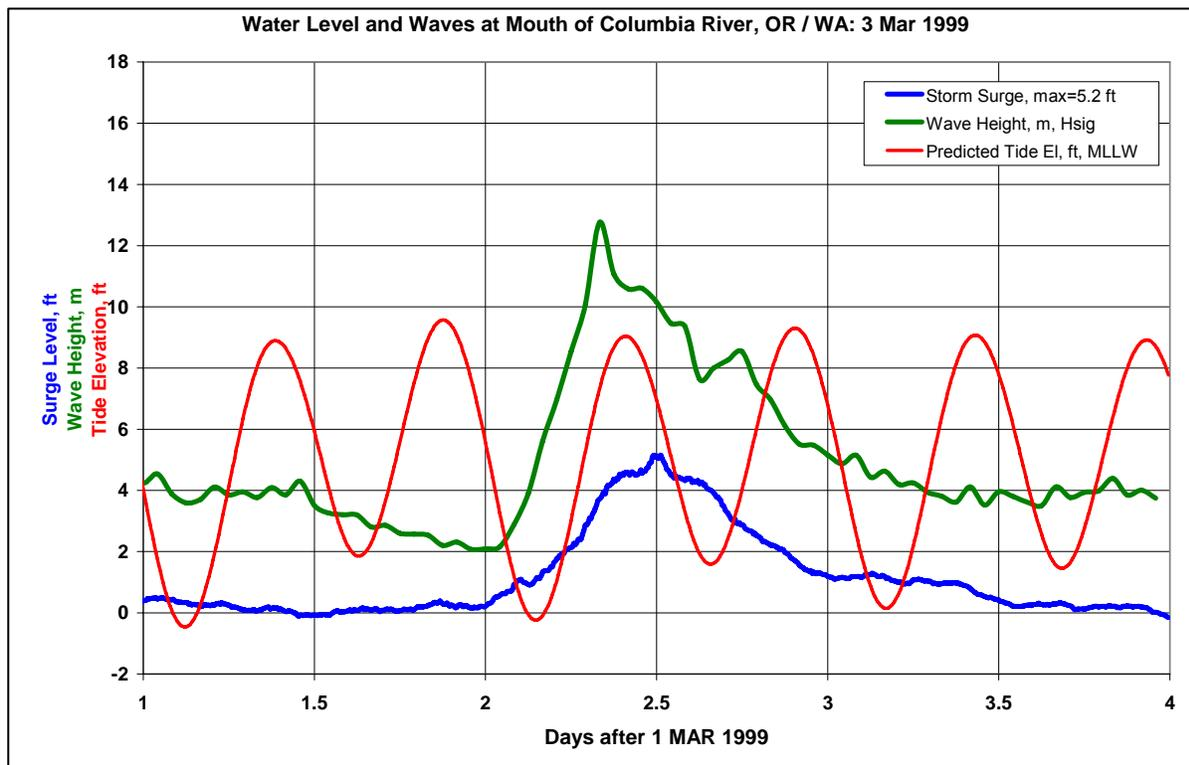
Figure 1. Examples of wave conditions and water levels that affect the coastal margin during extreme storm events. Storm surge = observed water elevation – predicted tide elevation. Top panel is offshore LA: due to Hurricane Katrina (water level is from NOAA gage at SW Pass, waves are from NDBC 46040). Bottom panel is offshore OR / WA: due to an extreme extratropical low pressure system (water level is from NOAA gage at Toke Pt. WA, waves are from NDBC 46029).
