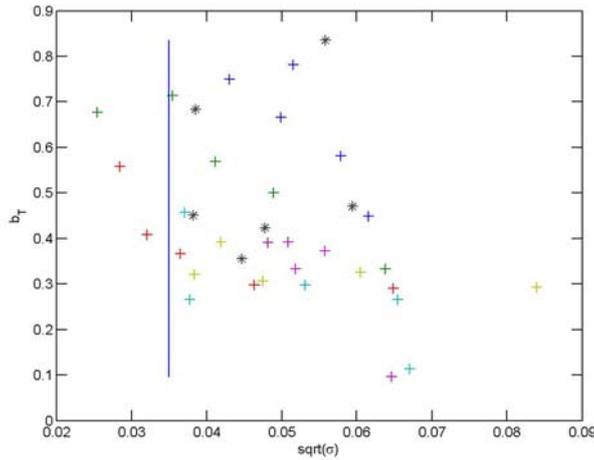
Figure 7. Breaking probability  $b_T(f)$  versus saturation parameter  $\sqrt{\sigma(f)}$ . Asterisks denote spectral peak points. Threshold 0.035 is shown with the solid line.
