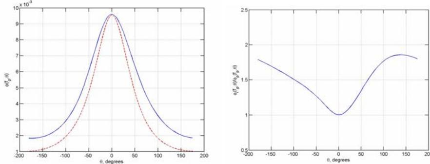
Figure 3. (left) Spectrum of breaking waves (blue) and broken waves (red); (right) Ratio of the two spectra.
