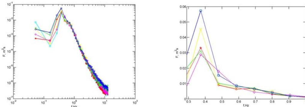
Figure 6. Wave spectra of Table 1. (left) Full spectra in log-log scale. (right) Spectra in  $f \approx 0.8f_p \div 3f_p$  range in linear scale.
