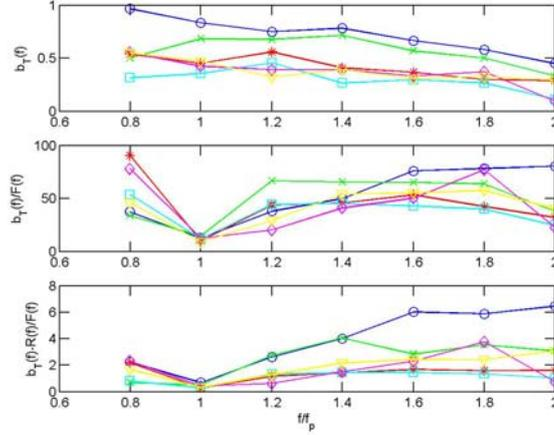
Fig. 5. Six wave records, see Table 1. (top panel) Breaking probability  $b_T(f)$  versus relative frequency. (middle panel)  $b_T(f)$  normalized by  $F(f)$ . (bottom panel) Product of bubble size  $R(f)$  and  $b_T(f)$ , normalized by  $F(f)$ .
