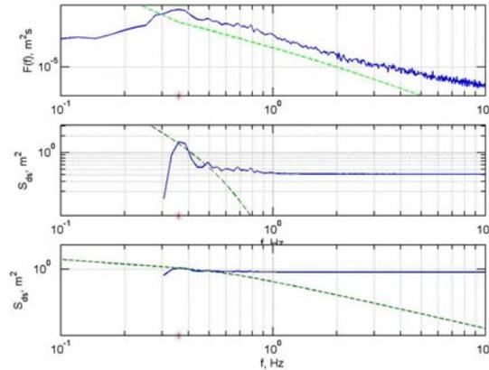
Figure 9. (top panel) Wave spectrum (No.1, Table 1) and dimensional spectral threshold (dashed line). (middle panel) Close up of the bottom panel. (bottom panel) Young & Babanin (2006), solid line, and Melville & Matusov (2002), dashed line, dissipation functions.
