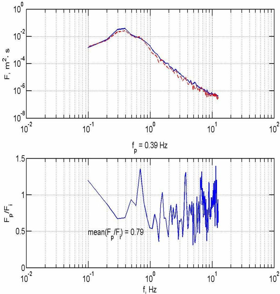
Figure 2. (top) Spectrum of breaking waves ( $F_p$ , blue) and broken waves ( $F_b$ , red dashed line); (bottom) Ratio of the two spectra.
