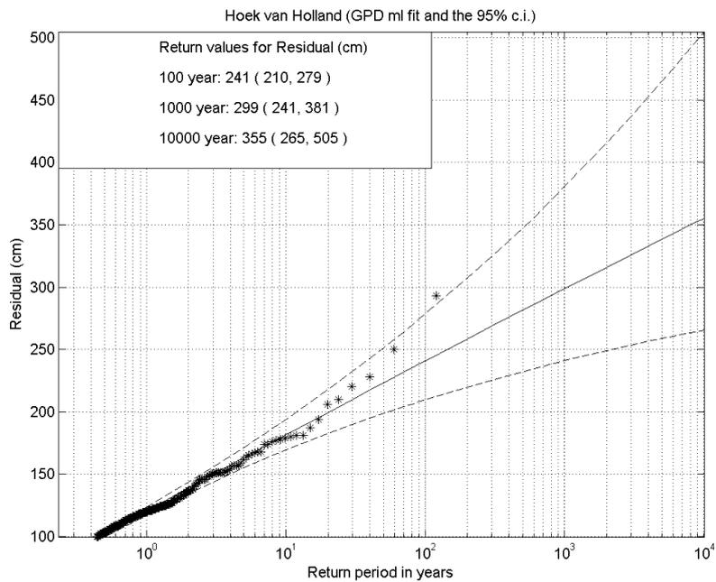
Figure 7 – Return value plot of the GPD fitted to the surge data obtained with the ML method (solid black line) and associated 95% confidence intervals (dashed black lines). The POT data are represented by the asterisks.
