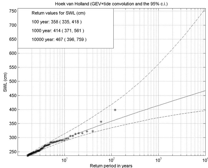
Figure 10 – Return value plot of the convolution of the astronomical tide and the AM surge levels (solid black line) and associated 95% confidence intervals (dashed black lines). The corresponding SWL AM data are represented by the asterisks.
