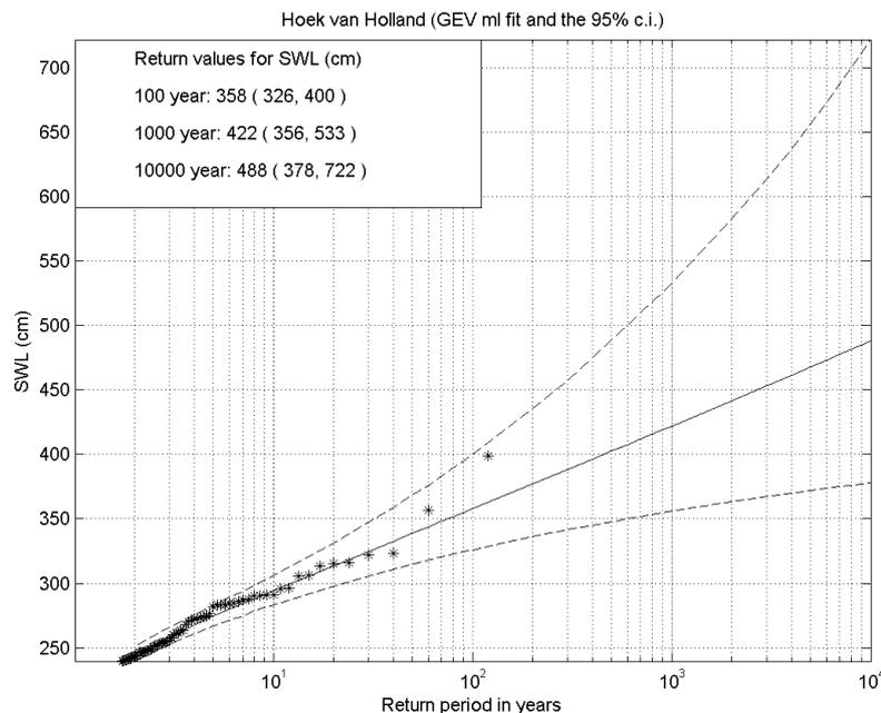
Figure 5 – Return value plot of the GEV fitted to the SWL data obtained with the ML method (solid black line) and associated 95% confidence intervals (dashed black lines). The AM data are represented by the asterisks.
