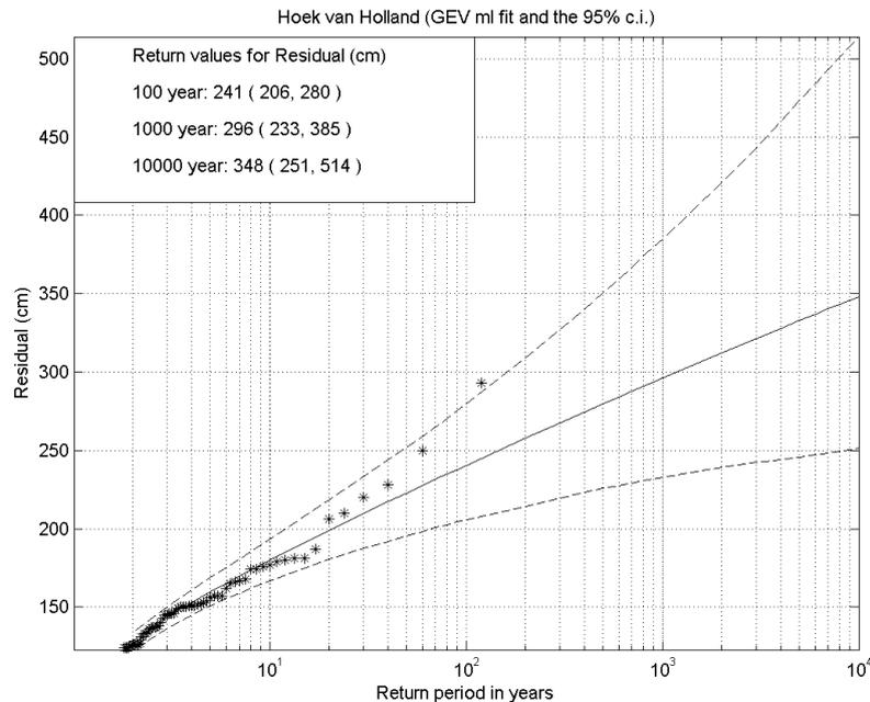
Figure 9 – Return value plot of the GEV fitted to the surge data obtained with the ML method (solid black line) and associated 95% confidence intervals (dashed black line). The surge data are represented by the asterisks.
