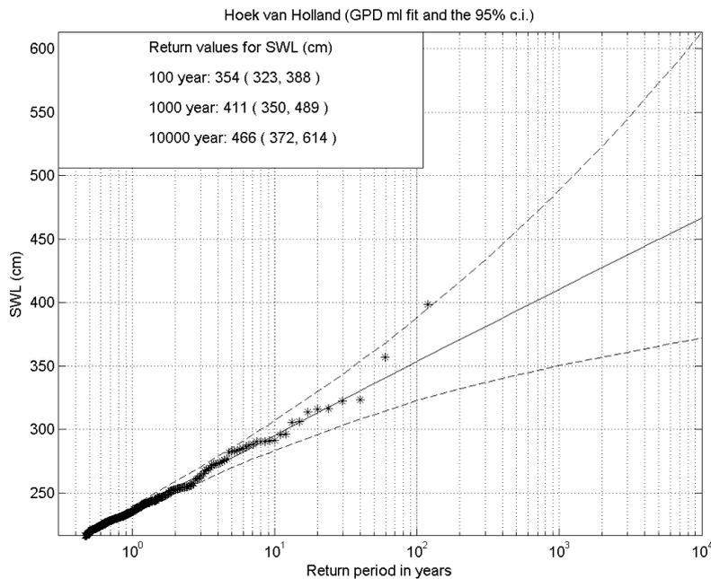
Figure 4 – Return value plot of the GPD model fitted to the SWL data obtained with the ML method (solid black line) and associated 95% confidence intervals (dashed black lines). The POT data are represented by the asterisks.
