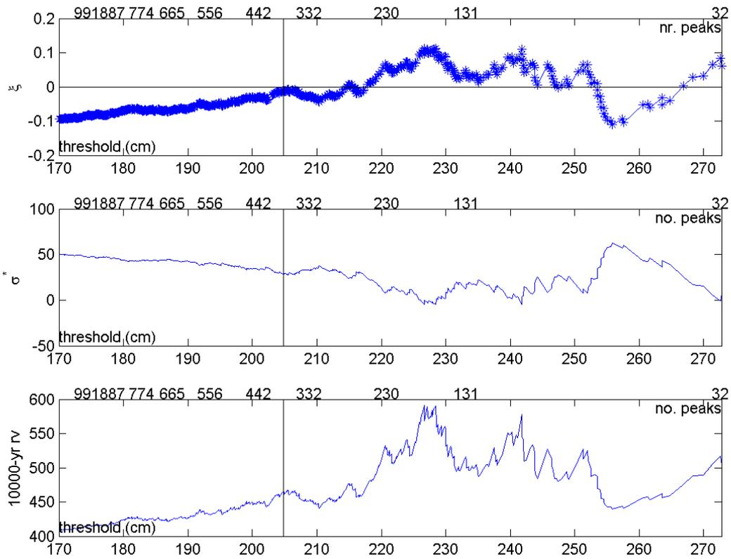
Figure 3 – Variation of the estimates of  $\xi$ ,  $\sigma^*$  and 1/10000 years SWL return values of the GPD model with the threshold used to collect the SWL POT sample.
