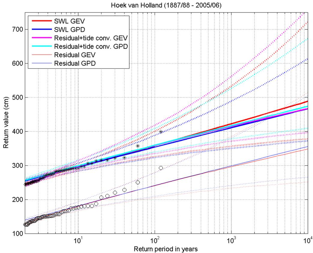
Figure 11 – Return value plot constructed with the results from all the analyses, including 95% confidence bands as dashed lines. The SWL data are represented by the asterisks and the surge data by the circles.
