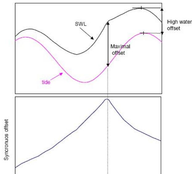
Figure 2 –Schematic representation of high water offset and synchronous offset.
