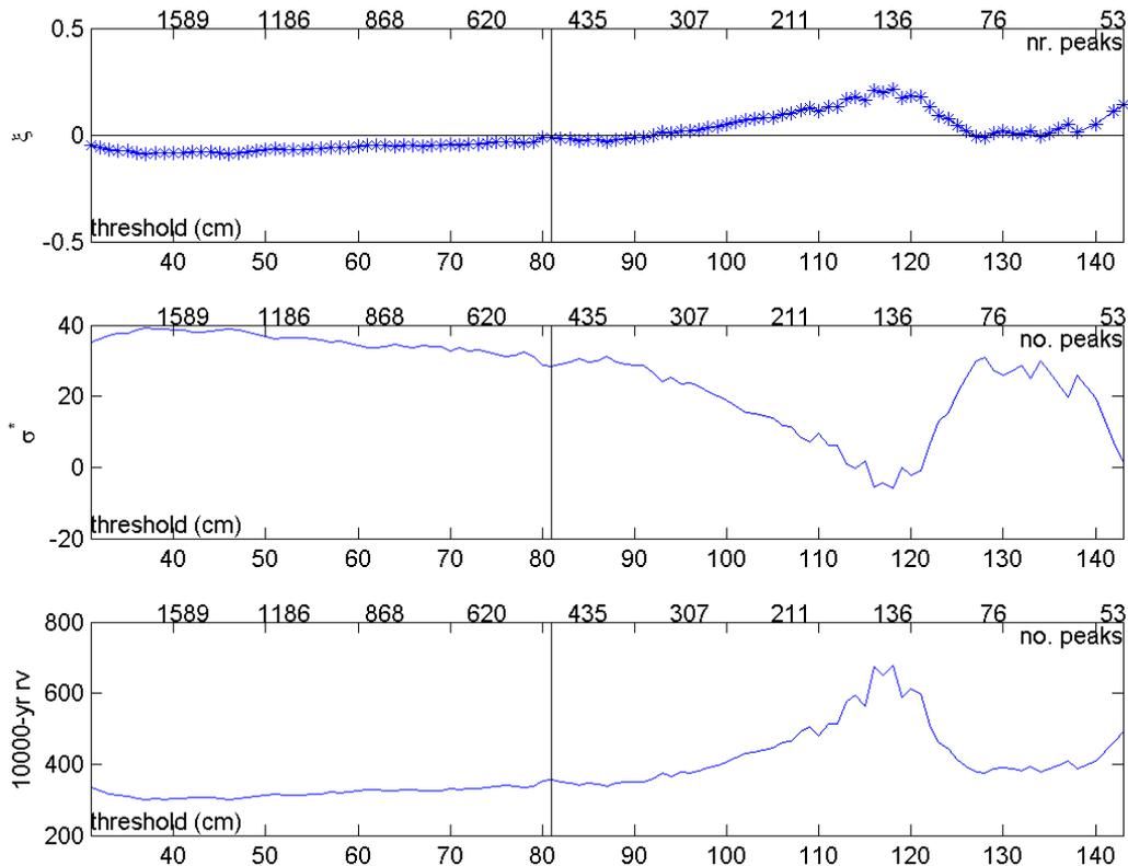
Figure 6 – Variation of the estimates of  $\xi$ ,  $\sigma^*$  and 1/10000 years surge return values of the GPD model with the threshold used to collect the surge POT sample.
