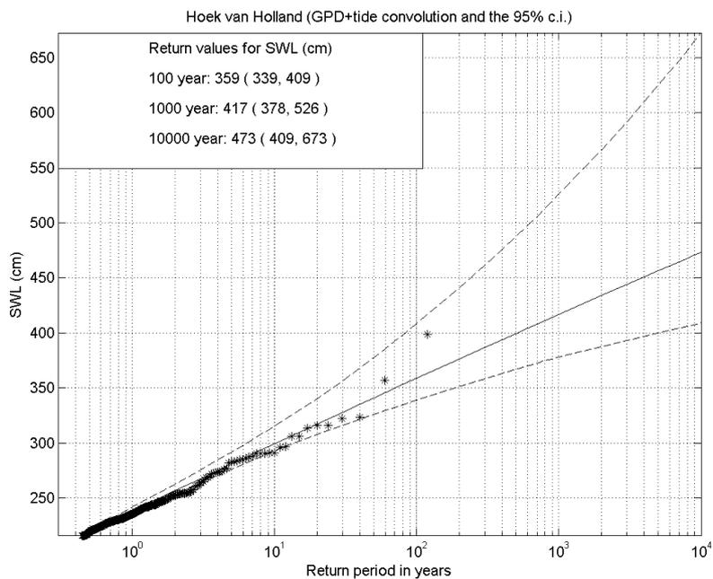
Figure 8 – Return value plot of the convolution of the astronomical tide and the surge levels (solid black line) and associated 95% confidence intervals (dashed black lines). The corresponding SWL data are represented by the asterisks.
