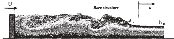
Figure 3: Sketch of the bore generated by a piston moving horizontally with velocity U in a layer of fluid with initial depth h_0 .
